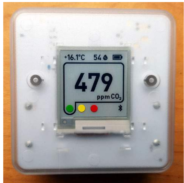
Figure 4. CO 2 monitor (Aranet4) with traffic light indication.
