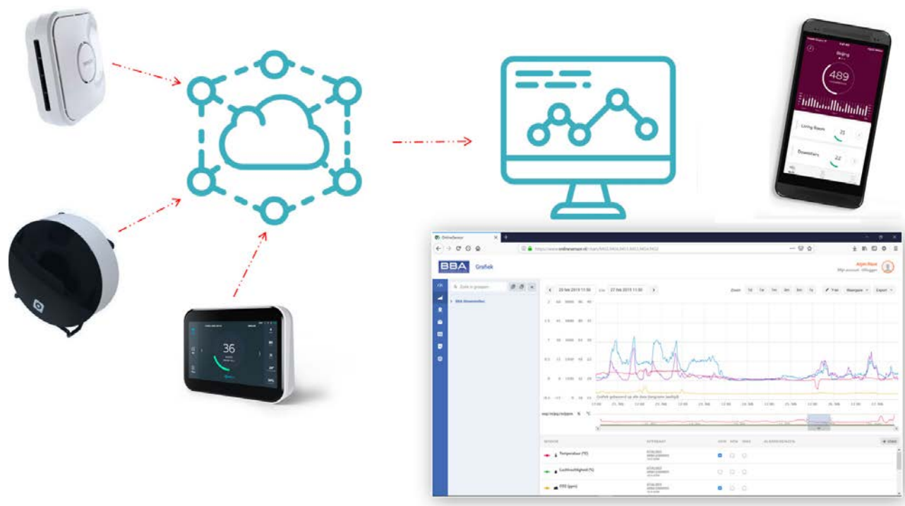
Figure 3. Core elements of an IEQ sensor network.
